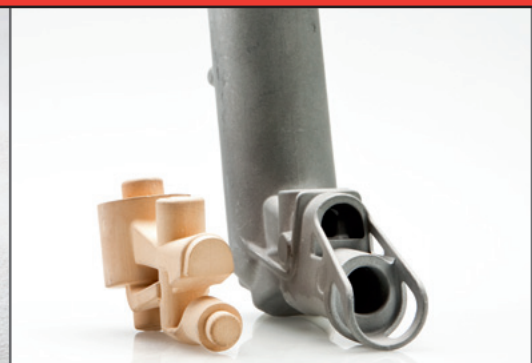
Complex core for internal shape of a high pressure pistol, core dimensions app. 70 x 45 mm
