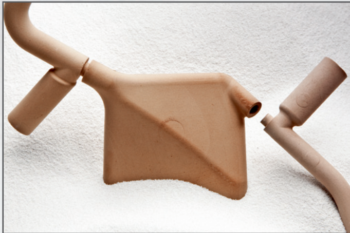
Complex internal shape, realized with plug-connection-techniques
