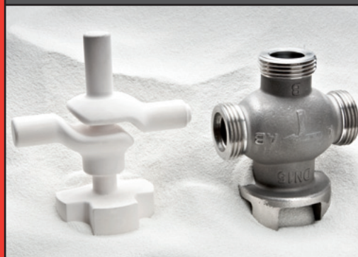
Ceramic core for Valve-body height 120 mm
