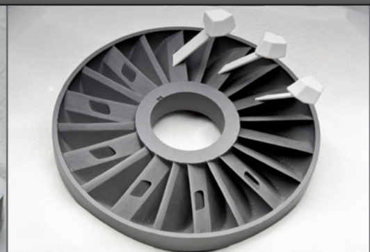
Stator for Voith-Retarder Ø 200 mm slot-thickness from ceramic core 2.5 mm
