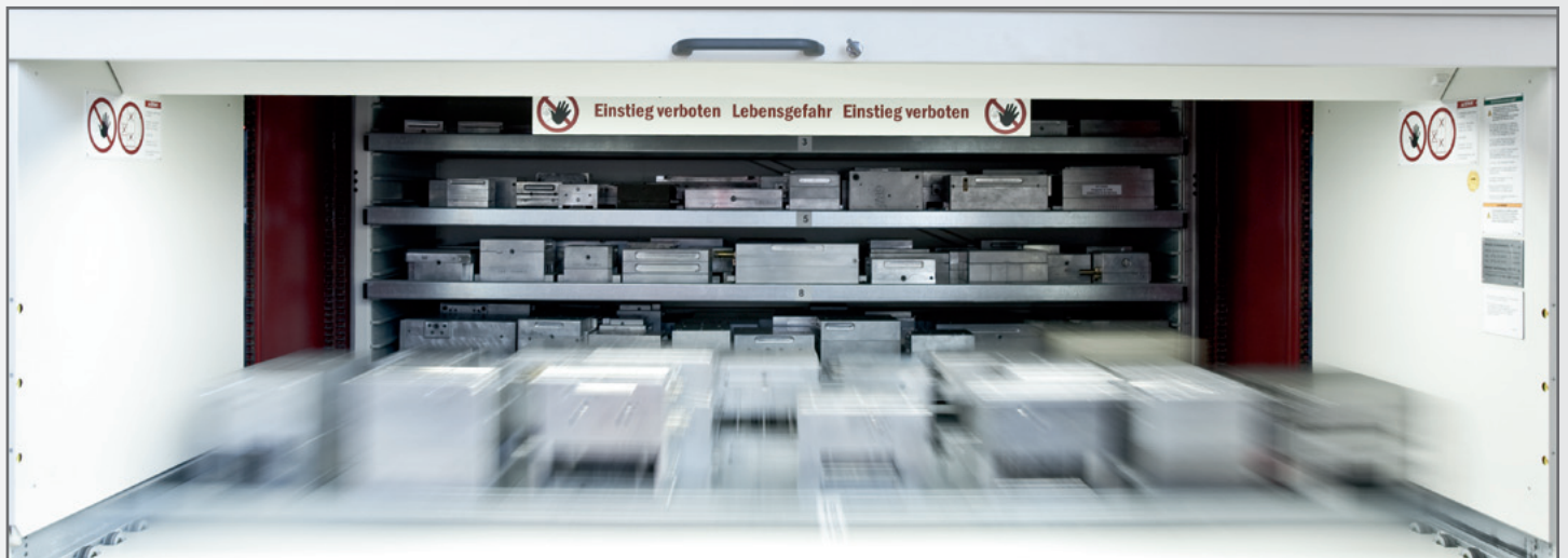
Modern „lean-lift“ stock system for tools
